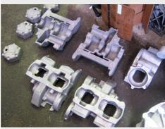
Cast engine casings ready for machining
